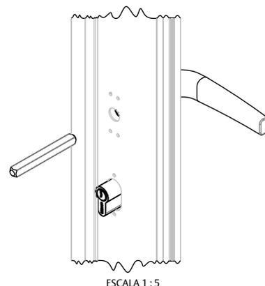
**PASSO 4:** ENCAIXE A OUTRA MAÇANETA MAC EURO NA HASTE, FIXE COM OS PARAFUSOS AUTOATARRAXANTES E GIRE A CAPA. FIXE A BASE DA ROSETA E CLIQUE A CAPA.
