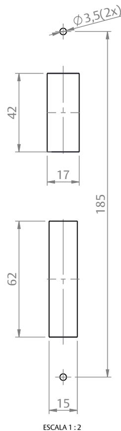
\*USINAGEM (REFILE) DA TESTA DA FECHADURA: FAZER ESSA USINAGEM (REFILE) NO MATA JUNTA APENAS QUANDO A FECHADURA FOR APLICADA EM PERFIS DA LINHA 25.
