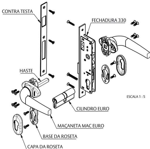
**PASSO 1:** COM A FECHADURA 330, O CILINDRO EURO E A CONTRA TESTA JÁ INSTALADA, FIXAR UMA DAS MAÇANETAS MAC EURO EM UM DOS LADOS DO PERFIL COM OS PARAFUSOS AUTO-ATARRAXANTES. FAZER O MESMO COM UMA DAS ROSETAS, FIXAR A BASE E DEPOIS DISSO, CLICAR A CAPA.
