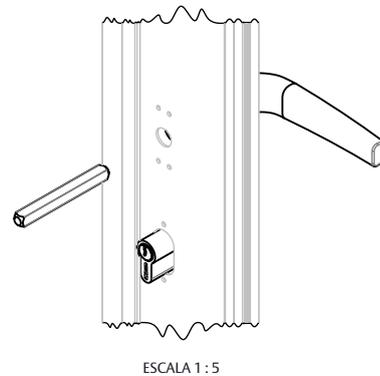
**PASSO 4:** ENCAIXAR A OUTRA MAÇANETA MAC EURO NA HASTE, FIXAR COM OS PARAFUSOS AUTO-ATARRAXANTES E GIRAR A CAPA. FIXAR A BASE DA ROSETA E DEPOIS DISSO, CLICAR A CAPA.
