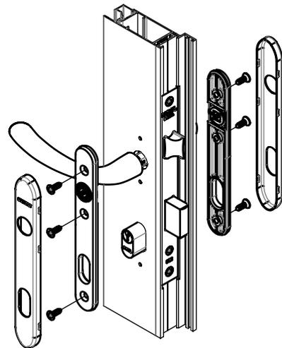
5. APÓS A USINAGEM DO MARCO (VER CATÁLOGO DA CONTRATESTA 295), POSICIONAR CONTRATESTA (VENDIDO SEPRADAMENTE) E FIXAR COM PARAFUSOS ALLEN SEM CABEÇA.
