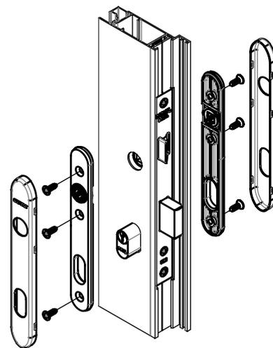
5. APÓS A USINAGEM DO MARCO (VER CATÁLOGO DA CONTRATESTA 295), POSICIONAR CONTRATESTA (VENDIDO SEPRADAMENTE) E FIXAR COM PARAFUSOS ALLEN SEM CABEÇA.
